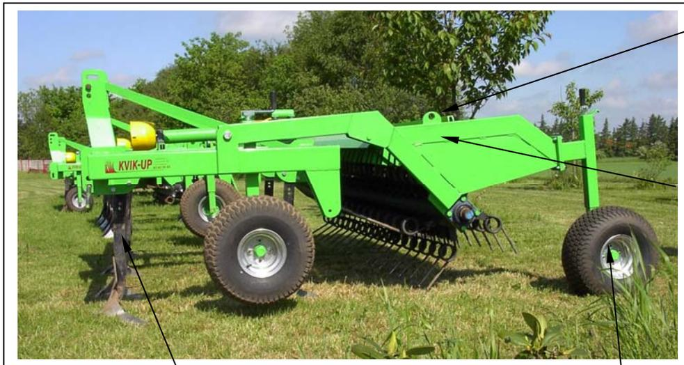
Adjust the wheels so that the teeth sticks approx. 5-15 centimeters in depth. The harrow must run partly on the tractor's lift system so that the harrow's wheels touch the earth vaguely.
